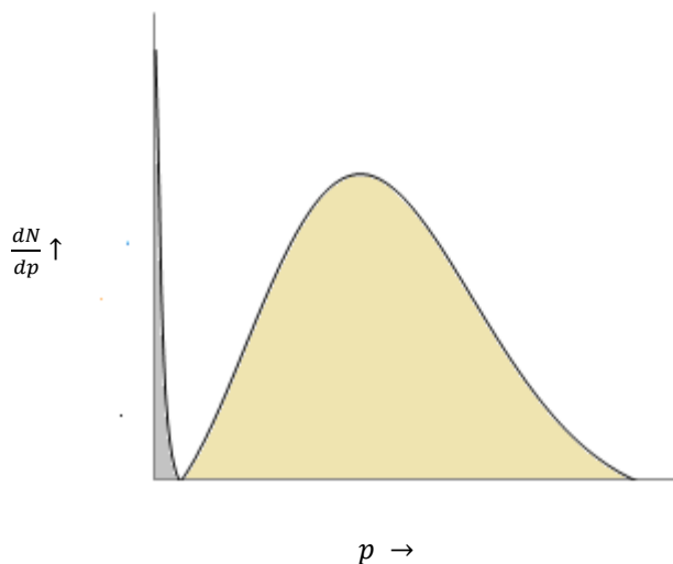
Figure 2 Momentum distribution of Bose particles in an ideal Bose gas below T < T_c , Grey area under the delta function shows the condensate contribution.
